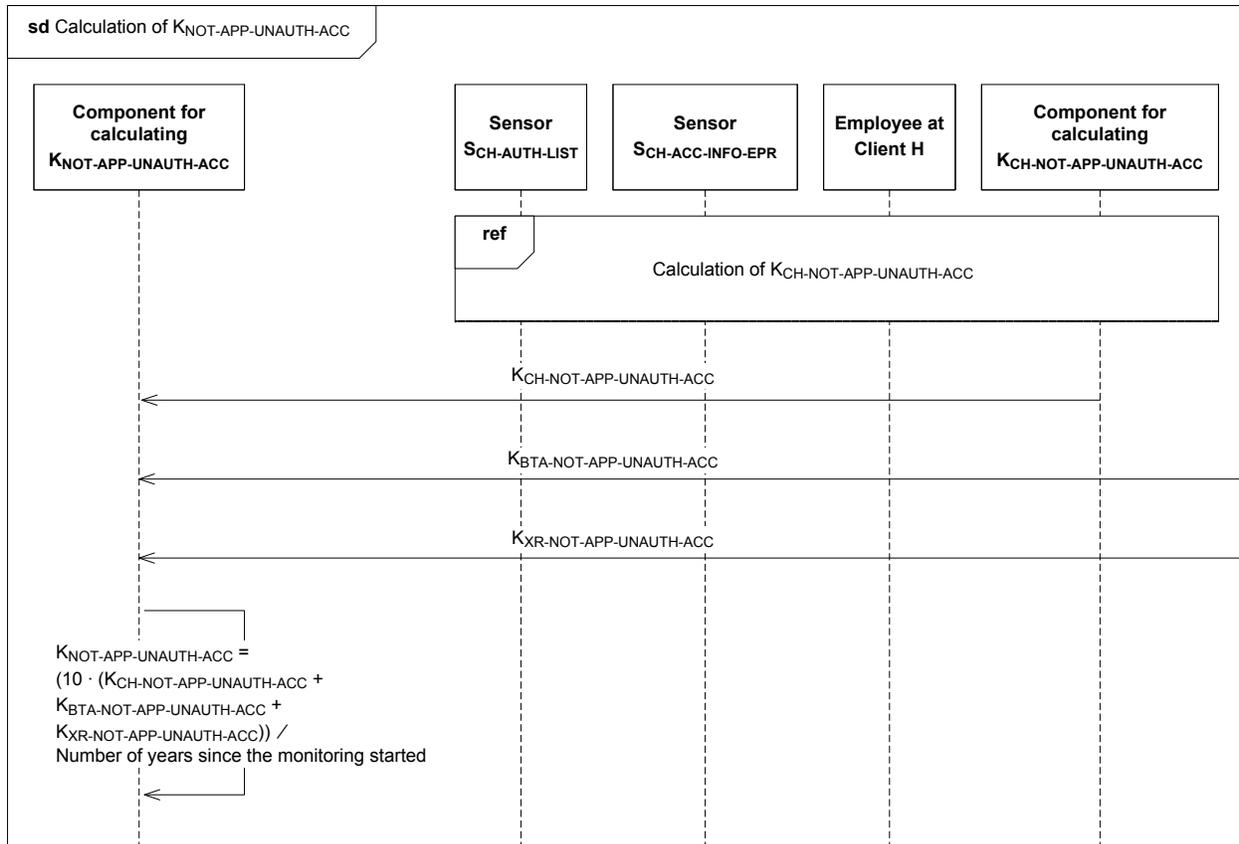
Figure 7. The sequence diagram “Calculation of  $K_{NOT-APP-UNAUTH-ACC}$ ”
