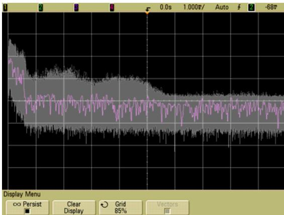
Figure 3: Long-term spectral analysis of stereo-signal from NRK P1 (128 kbit/s). x: 5 kHz/div., y: 20 dB/div.
