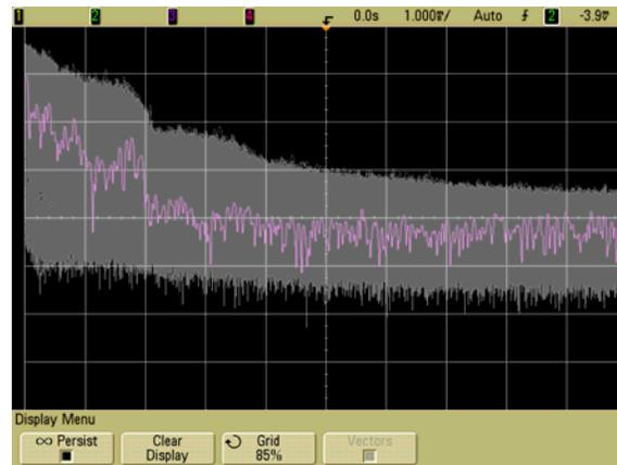
Figure 1: Long-term spectral analysis of mono-signal from Moox Live (80 kbit/s). x: 5 kHz/div., y: 20 dB/div.
