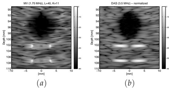
**Fig. 6.** Simulated cyst phantoms using a 18.5 mm, 96 element transducers. (a) MV (1.75 MHz,  $L = 40$  and  $K = 11$ ). (b) DAS (3.5 MHz). Tx focus was 100 mm.
