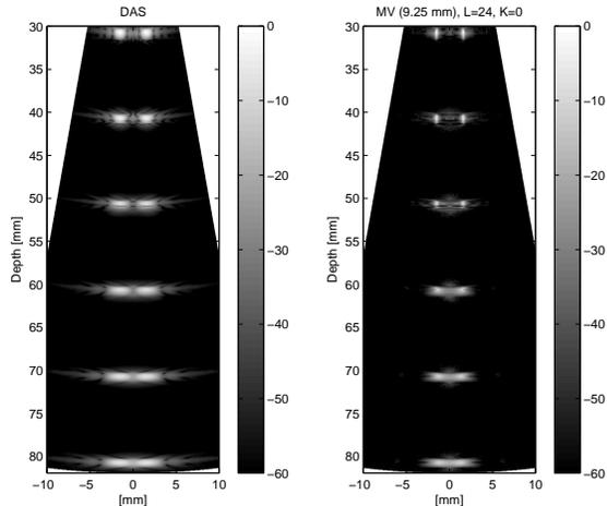
**Fig. 3.** Simulated wire targets, 3.5 MHz, dynamic Tx and Rx focus. Left: DAS using 96 element, 18.5 mm transducer, rectangular window. Right: MV using 48 element, 9.25 mm transducer.
