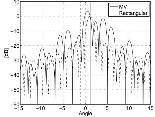
**Fig. 2.** Beam pattern of the MV beamformer for two wire targets. The dashed line is the beam pattern of a rectangular window. The vertical lines indicate the wire targets, and the solid line is the steering angle.
