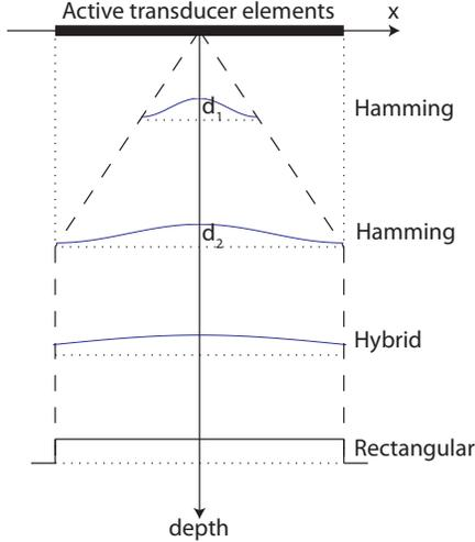
**Fig. 1.** Dynamic aperture and dynamic weighting as typically used in medical ultrasound
