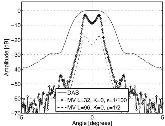
**Fig. 4.** Response of DAS (solid), MV with heavy diagonal loading, but no subarray averaging (dashed) and MV with subarray = 32 and a small amount of diagonal loading (solid, diamonds) for two wires at 70 mm.
