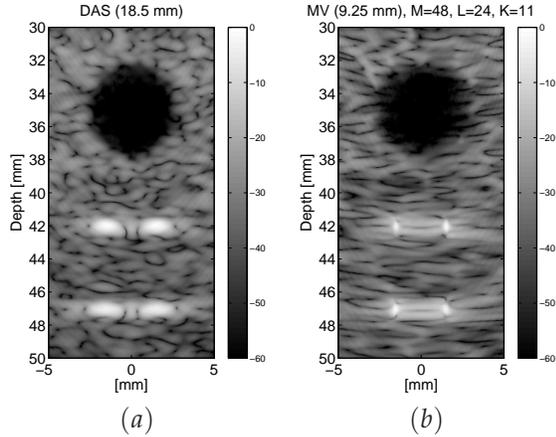
**Fig. 5.** Simulated cyst phantoms using 3.5 MHz transducers. (a) DAS with 96 element, 18.5 mm transducer (rectangular window) (b) MV with 48 element, 9.25 mm transducer ( $L = 24$  and  $K = 11$ ). Tx focus was 35 mm.
