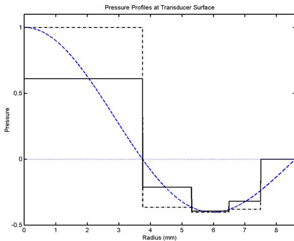
**Figure 1** Pressure profiles : Ideal Bessel (curved), Mean quantised (solid), Maximum quantised (dashed)
